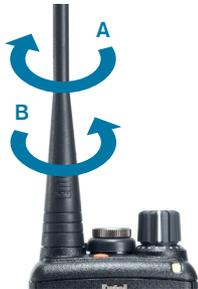
1. To attach, carefully align the antenna with the socket. Screw in the antenna clockwise (taking care not to cross the thread) until it is seated firmly with the accessory cover's rubber ring between the antenna and the top of the radio (A).
