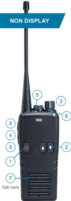
1. On/Off button: press and hold to turn the radio on or off.
