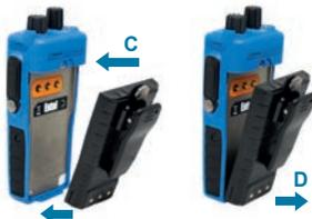
1. To attach, locate the pegs on the bottom of the battery into the slots on the radio and press the top of the battery against the radio. Secure battery by tightening the screw clockwise by hand (do not use any implement or over tighten) (C).
