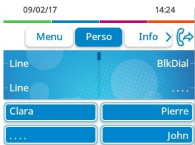
User interface with virtual add-on. 4 programmable softkeys are displayed and can be used as a smart add-on module.
