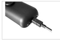
Plug the USB cable into the USB port of your phone. The other end of the USB cable can be plugged into the AC/DC adaptor or into a computer USB port.
