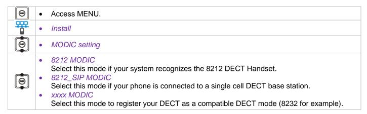
During registration phase, to improve security and optimize registration in a multi-system environment, the handset enforces a minimum signal strength level to accept to register to a base station. To achieve the conditions, it is recommended to perform registration in a place where a base station is in direct visibility within a 20 m range. If base station is not visible the range shall be lowered.
